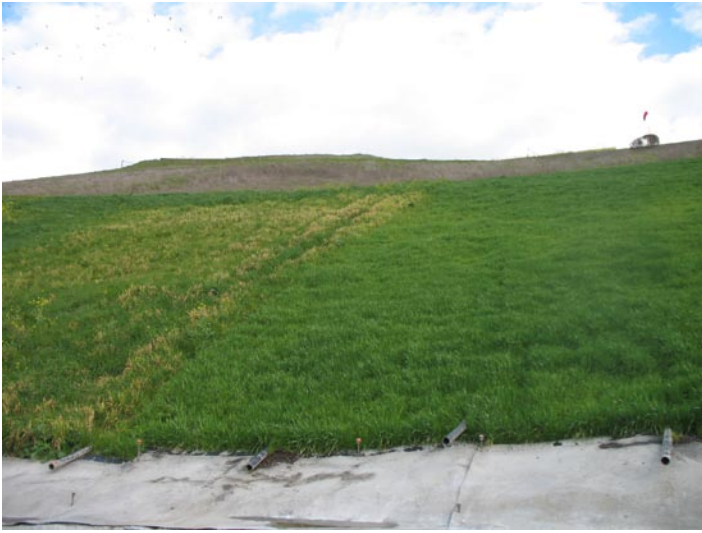
February 12: Area of compost (on the right) very green. Area of hydroseeding (on the left) beginning to yellow.
